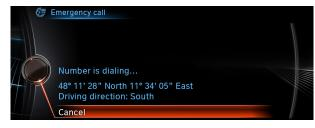
Automatic activation as soon as crash sensors or airbags are triggered.
