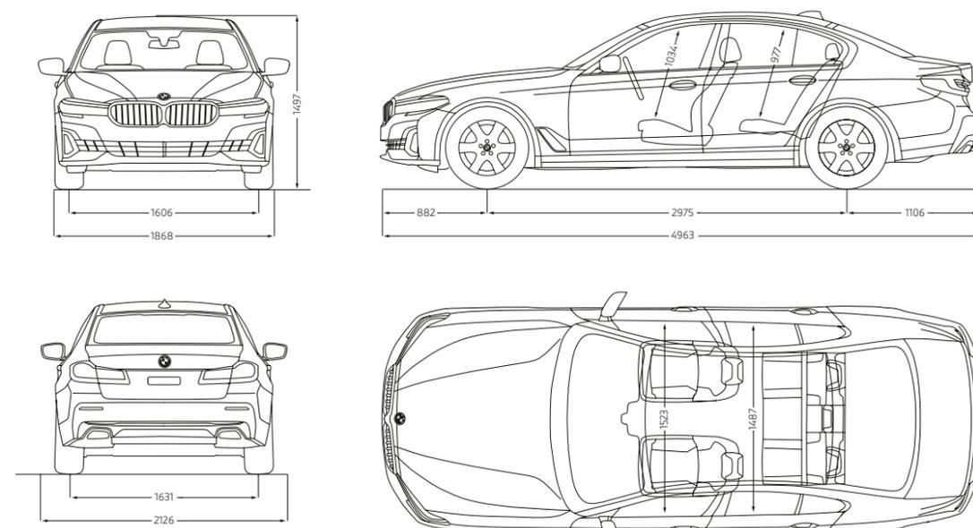
All dimensions in the technical drawing are given in millimetres. The dimensions for M550i xDrive may vary.
