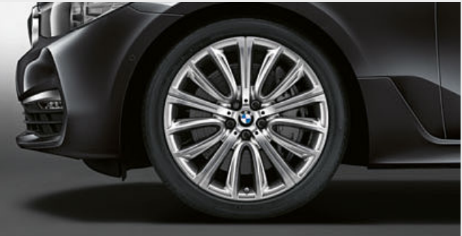
□ 20" light alloy wheels V-spoke style 628 Bicolour with mixed tyres and run-flat properties, front 8.5J x 20 with 245/40 R20 tyres, rear 10J x 20 with 275/35 R20 tyres.
