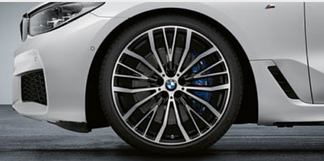
○ The premium-quality 21" light alloy wheels V-spoke style 687 are designed in Bicolour Black, gloss-lathed on the visible side, and feature a weight-optimised, rolled-steel rim bed. Summer complete wheel set with run-flat mixed tyres, wheel size 8.5J x 21 with tyre size 245/35 R21 96Y XL RSC at the front and 10J x 21 with tyre size 275/30 R21 98Y XL RSC at the rear.
