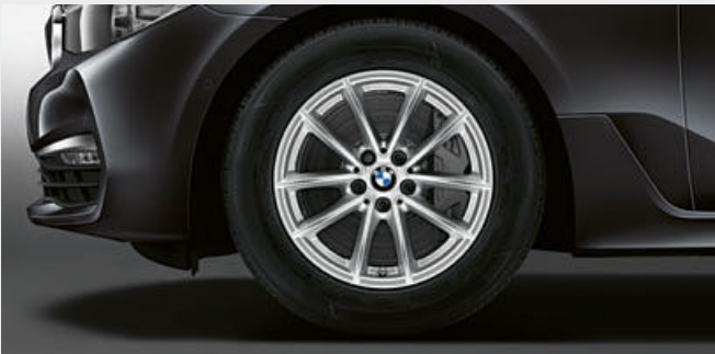
■ 17" light alloy wheels V-spoke style 618, 7.5J x 17 with 225/60 R17 tyres.
