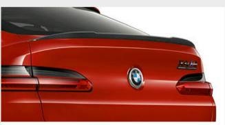
☐ The M specific carbon-fibre rear spoiler provides more contact pressure on the rear axle at higher speeds. At the same time, it lends the rear view characteristic sportiness and promises highly dynamic driving experiences.3
