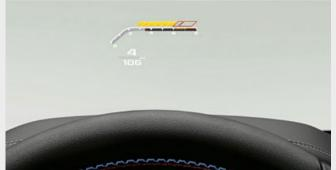
☐ The full-colour BMW Head-Up Display¹ incl. M specific display projects information relevant to the journey directly into the driver's field of vision, thereby allowing them to fully concentrate on driving. Information such as the current speed and, depending on the equipment, navigation directions, Speed Limit Info including no-overtaking indicator, along with telephone and entertainment lists are displayed.
