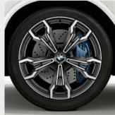
☐ 21" M light alloy wheels V-spoke style 765 M Bicolour Orbit Grey with mixed tyres, gloss-lathed, front 9.5J x 21 with 255/40 R21 tyres, rear 10J x 21 with 265/40 R21 tyres.
